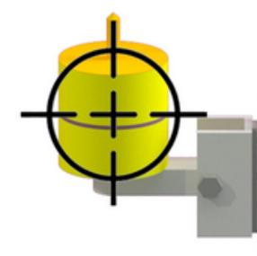
1. Adjust the instrument constant to +25.9 mm (offset + 25.9mm).
